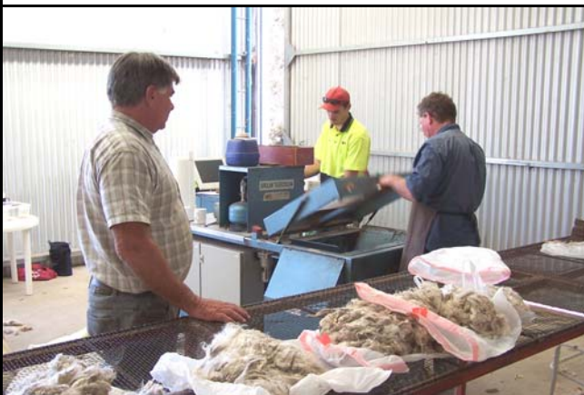
Whole fleeces are sampled using 6 mini cores taken from the compressed fleece
